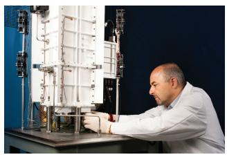
An engineer works on an engineering test unit of the ASRG. Such test units (with non-nuclear heat sources) have operated for a total of more than 33,000 hours in the laboratory over more than a decade of increasingly integrated development work.
