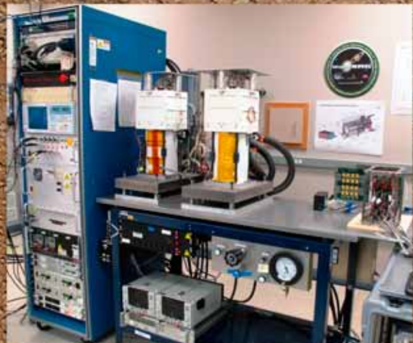
ASC-E2 #7 and #8 in Lockheed Martin Coherent Technologies controller testing.
