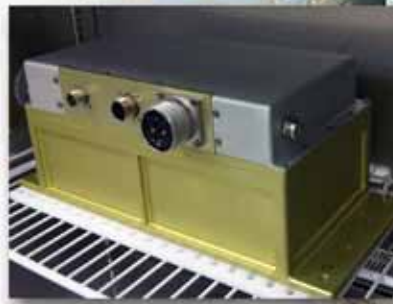
Battery unit (Ares 1).
