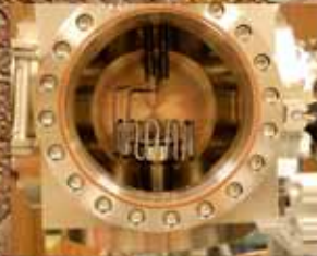
High-temperature heater head leak test rig.
